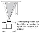
When the lens is shifted to leftmost. When the lens is shifted to rightmost.
